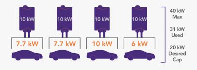
**With load balancing,** the maximum load is set at 20 kW. All four cars charge below their individual acceptance rates, making it easier to limit the overall consumption and manage demand charges.
